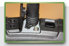
1/4 turn rotation to the left (counterclockwise) will seat the camlock connector properly into headset jack.
